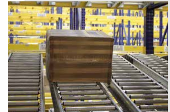
Full-width box support helps provide flow for damaged boxes.
