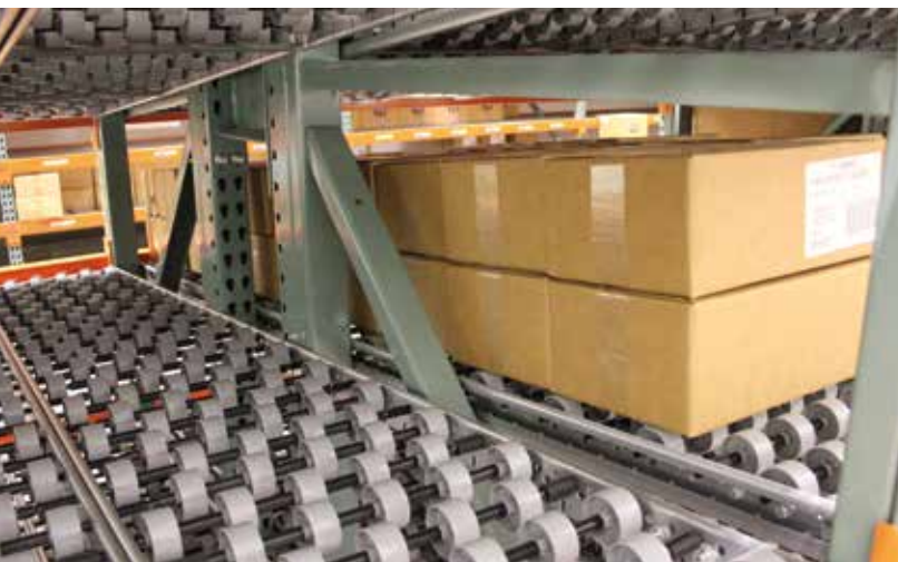
DISCHARGE END Adjustable end bracket rests in step of beam to allow beam to act as box stop.
