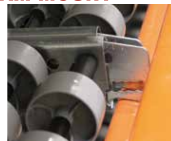
CHARGE END Heavy-duty end-bracket rests in step of beam and adjusts incrementally to adjust pitch for proper flow
