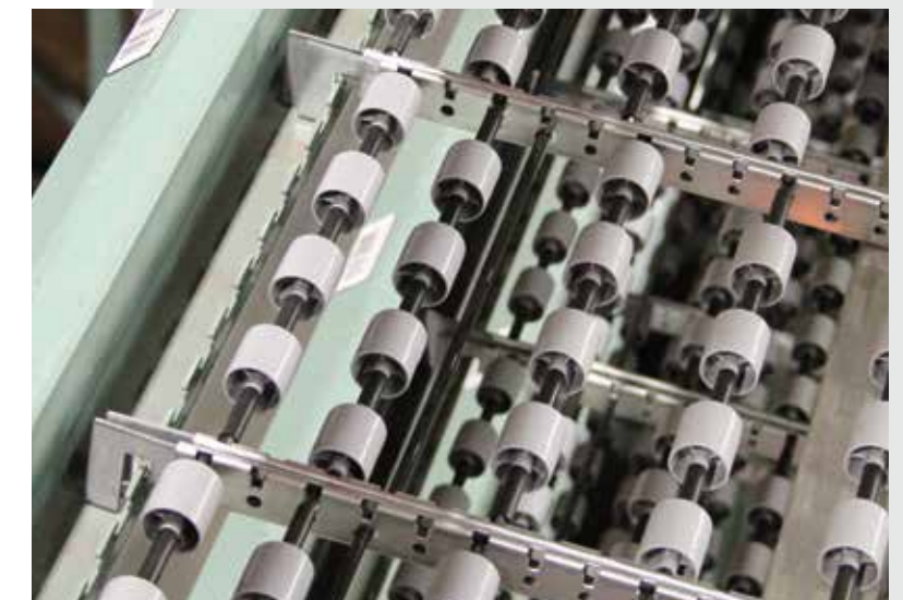
Entry and exit brackets mount into carton flow shelf members with no loss of clearance and no labeling disruption.
