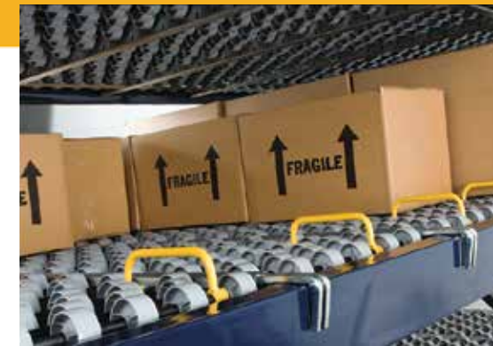
Dura-Flo Lane Indexers are easy to reposition.
