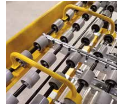
Lane indexers are easy to reposition.
