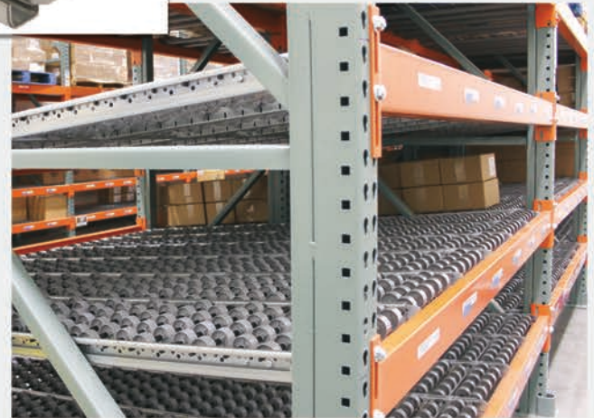
Contiguous wheel span creates a deck for mixed package width on the same shelf, maximizing space and efficiency.
