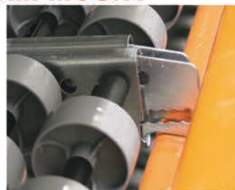
CHARGE END Heavy-duty end bracket rests in step of beam and adjusts incrementally.
