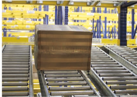
Full-width box support helps provide flow for damaged boxes.
