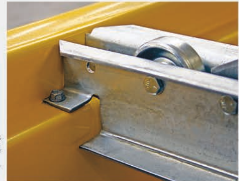
Metal skate wheel rails are notched to fit into the step of pallet rack beams.
