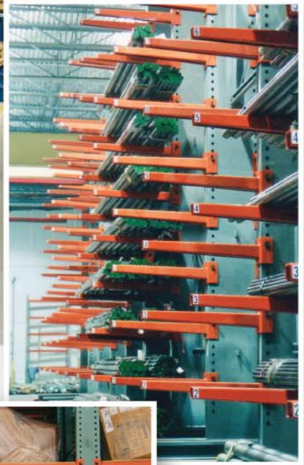
Pipe storage cantilever
