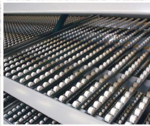
Carton Trax steel axle carton flow with UPICK knock-down modular shelves.
