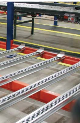
Pallet Flow used in pick module application with carton flow above
