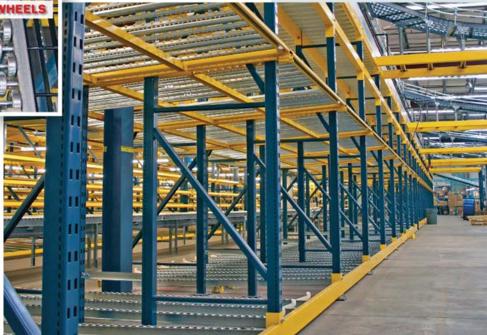
Pallet Flow used in pick module application with carton flow above
