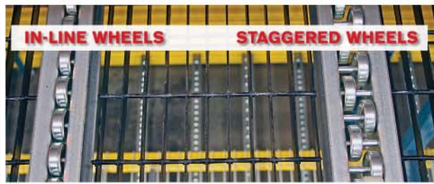
Staggered Wheels for heavier loads - 1 1/2" - 2" centers
