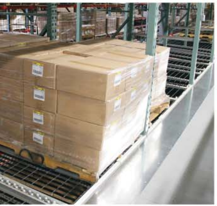
Pallets rest against pallet stop
