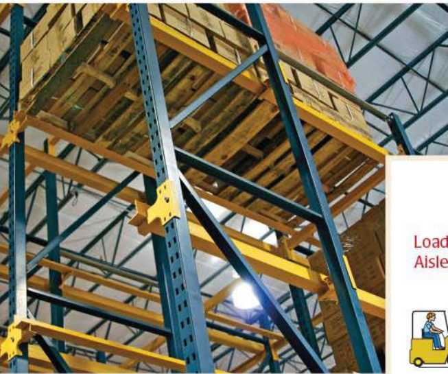
Pallets rest on rails within the bay.
