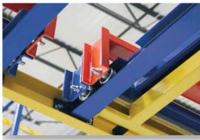
Carts flow automatically on four sealed wheels
