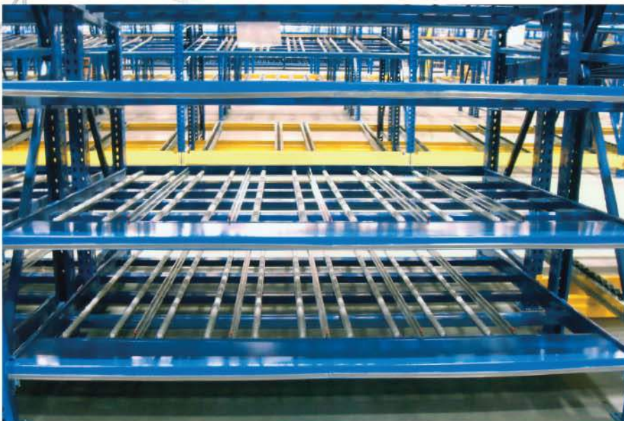
Optional impact deck helps prevent track damage.
